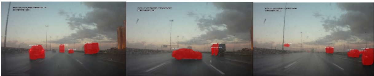
Figure 3.5 Detection results under a bad weather condition
