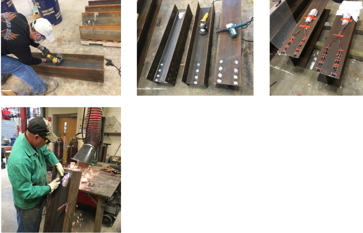
Figure B.1 Steel H-pile cleaning and strain gauges attaching
