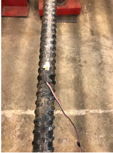
Figure 3.9 Installation of strain gauges on post-tensioned bar.
