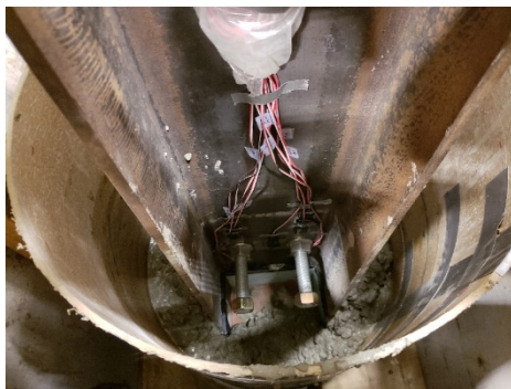
Figure B.7 CFRP jacket + HS specimen concrete placing
