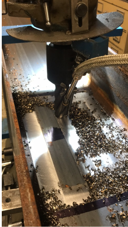
Figure B.11 Milling the webs to the reduced thickness
