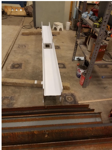
Figure B.12 Cleaning and painting the specimen with white water based paint
