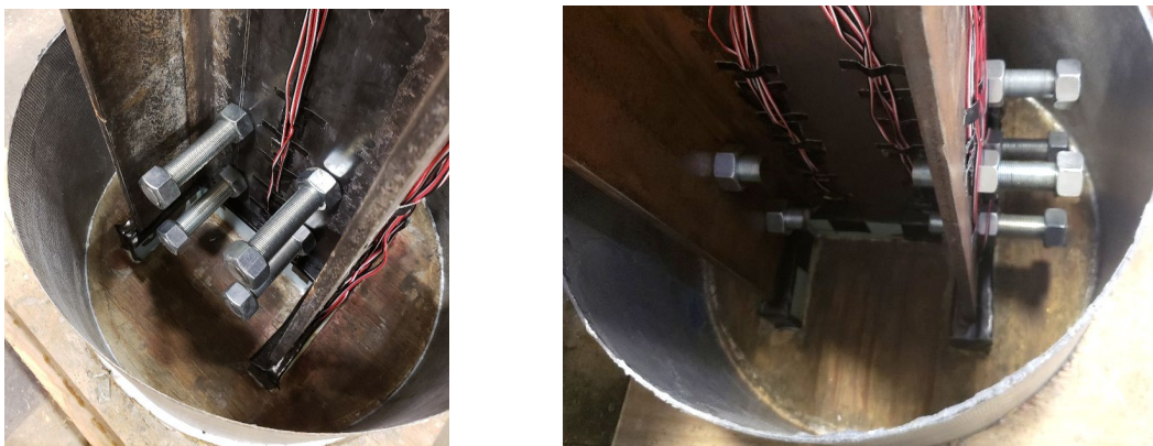
Figure 5.4 HS attached to web and flanges of the steel pile.
