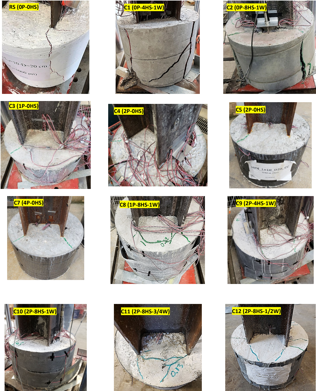
Figure 5.9 Failure modes of the test specimens.
