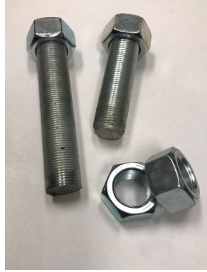
Figure 6.1 All threaded bars and heavy-duty nuts used as HSs.
