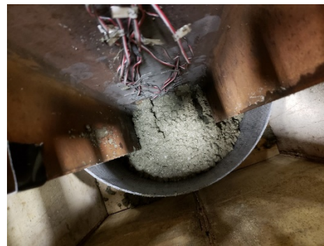
Figure B.7 CFRP jacket + HS specimen concrete placing
