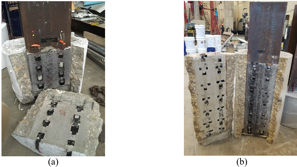
Figure 4.10 Concrete encasement – steel H-pile contact area condition (a) L_{CE} = 254 mm (10 in.), (b) L_{CE} = 508 mm (20 in.).
