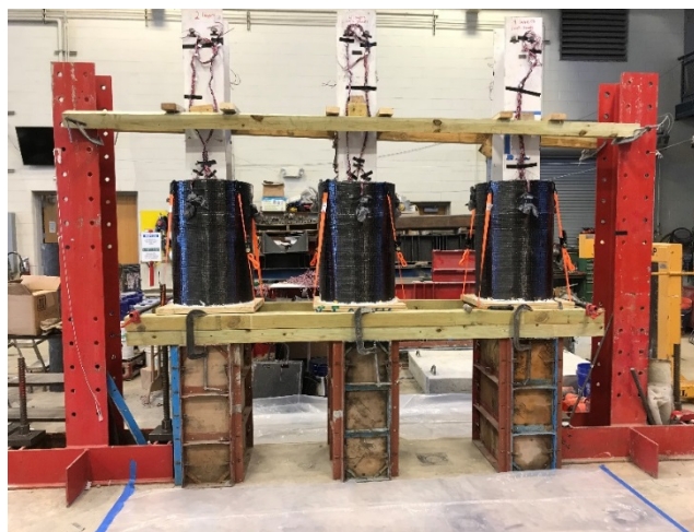
Figure 6.6 Specimens after CFRP Installation.
