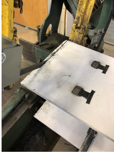
Figure B.13 Trimming the rough edges of the specimens
