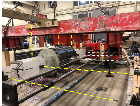
Figure 6.9 String potentiometer vertical and horizontal measurements.
