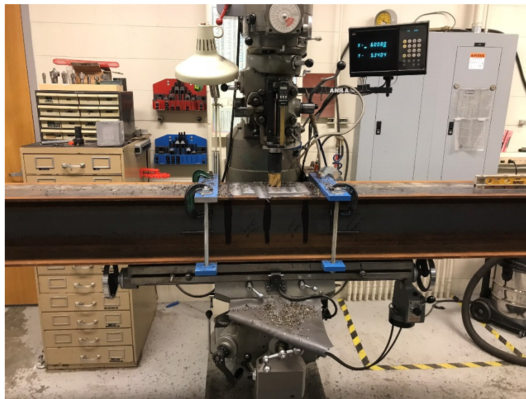
Figure B.10 Milling the flanges to the reduced thickness
