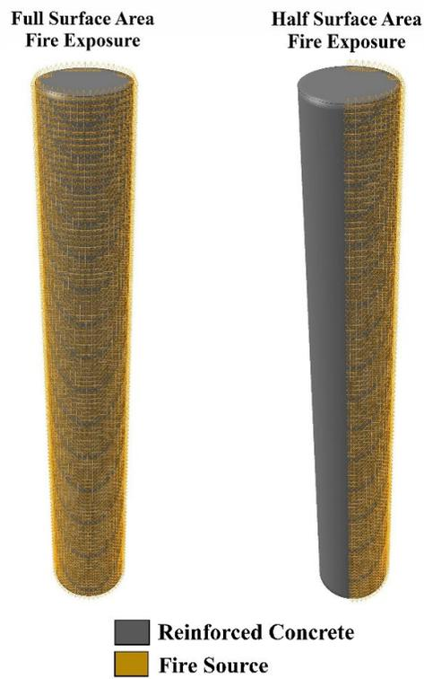
Figure 3.6 Full and half surface area fire exposure schemes
