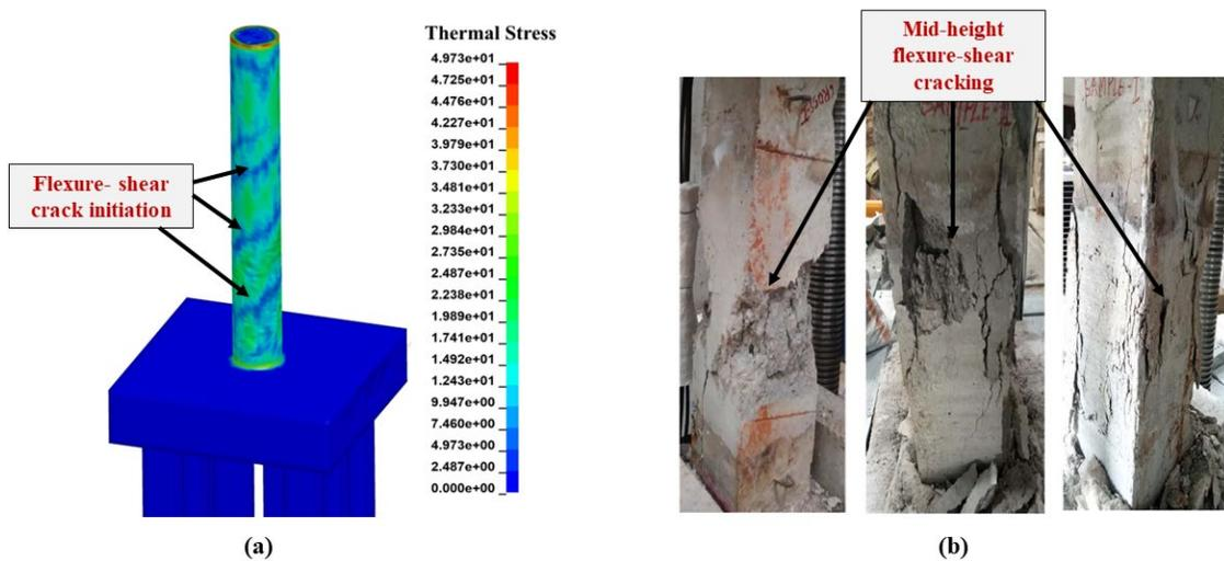
Figure 5.4 Effective thermal stress distribution and crack propagation: (a) FEM, 750 mm diameter, F90-I-B; (b) Experiment (Chinthapalli et al. 2019)
