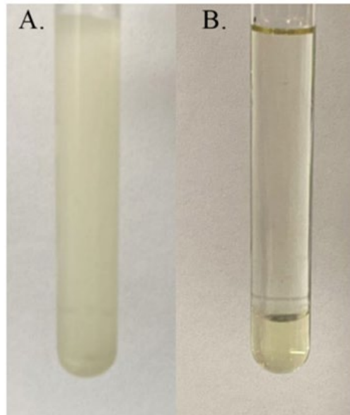
Figure 2.17 Emulsified fuel (10E5W) sample immediately a) after ultrasonication, and b) after phase separation [18].
